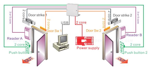
Gianni supplies all accessories for access control application including maglock, electric bolt lock, electric strike ,exit button, power supply, prox cards or fobs.
